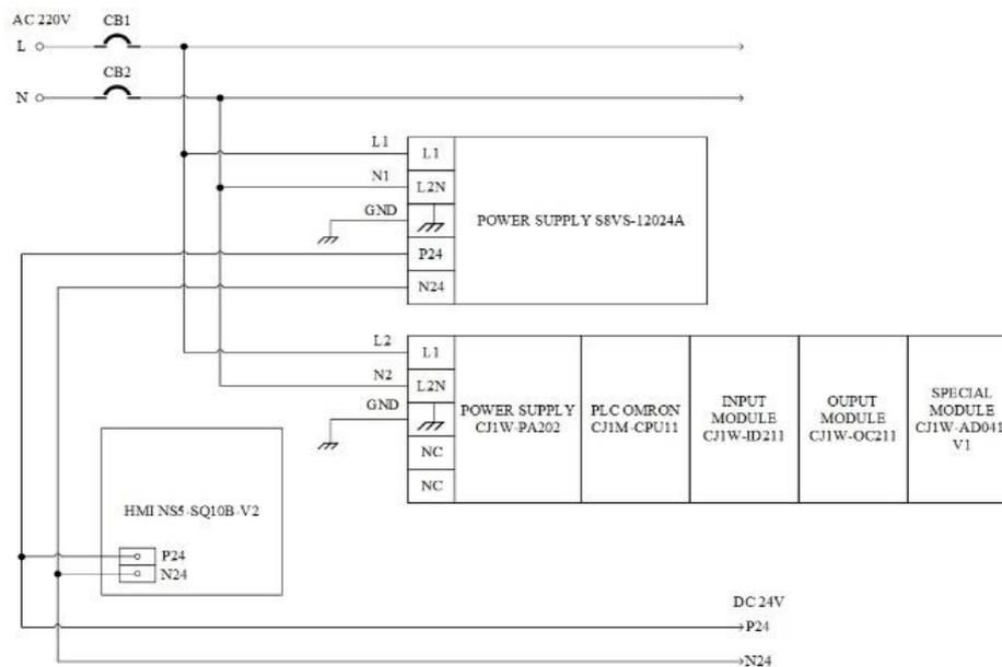
Fig. 3: Wiring of PLC, HMI, and power supply
