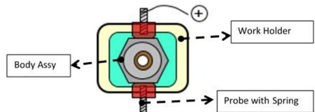
Fig. 3. The additional spring in jig
