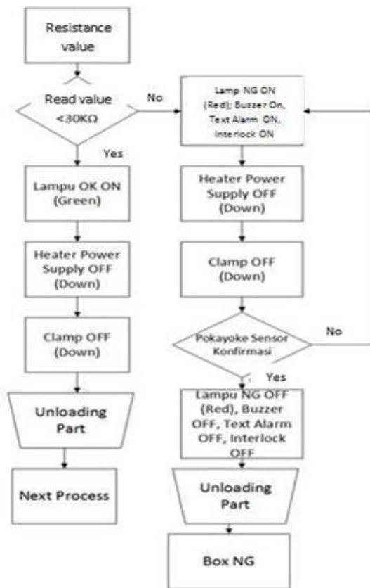
Fig. 4. The sequence of the flow chart
