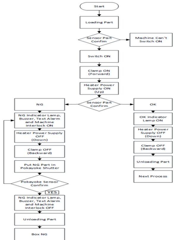
Fig. 2. Process flow operation of the function check machine
