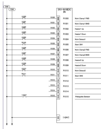
Fig. 10. Electrical wiring of photo electric sensor
