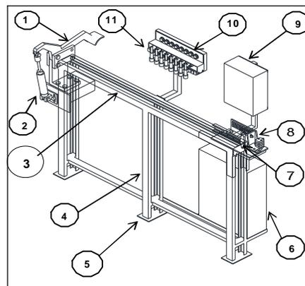
Figure 7. Design of Final Check machine and the parts
