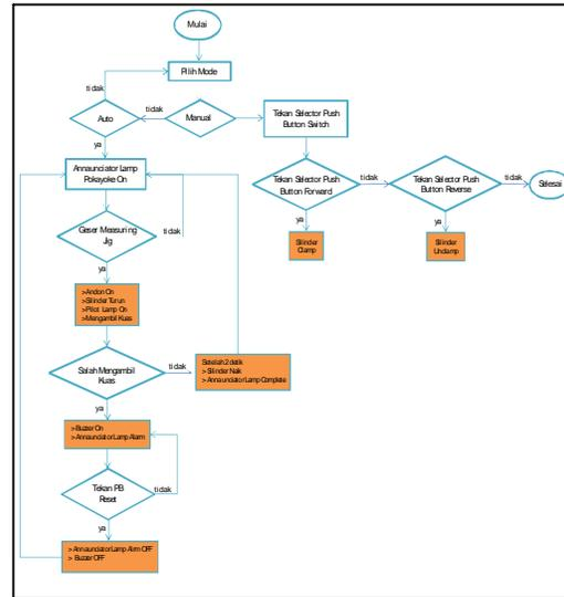
Figure 12. Flowchart of the Programming
