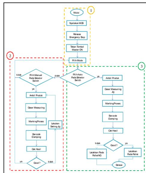
Figure 10. Flowchart of work sequence
