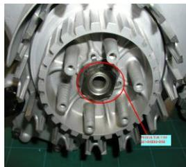
**Figure 1.** Coupling nut 261-04E06-00S on a motorcycle clutch
