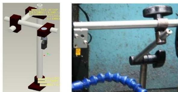
Fig 2. Design and realization of pokayoke sensor systems
