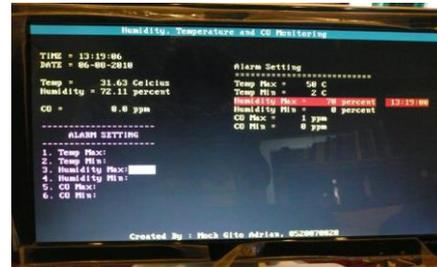
**Figure 15. Testing of LCD display**
