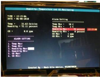
**Figure.13. LCD screen display monitor when the humidity reaches a maximum value**
