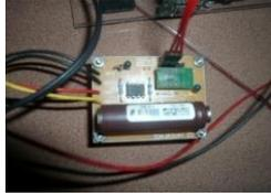
**Figure 4. Circuit of carbon monoxide (CO) sensor**
