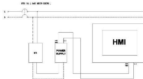
FIGURE 4. wiring power HMI curing machine
