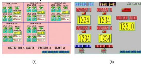
FIGURE 8. design layout HMI operator EBS (a) the display of the home screen, (b) display any curing machine
