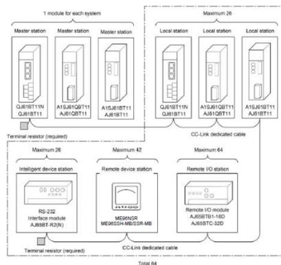
**FIGURE 1.** CC-Link configuration example
