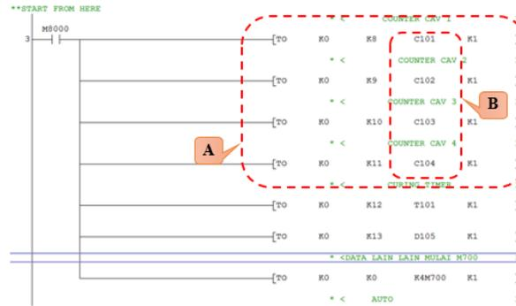
**FIGURE 9.** the program counter on PLC curing machine
