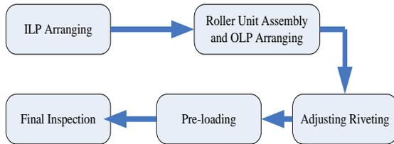
Figure 2. Assembling flow process of the cam chain in an assembly line LC
