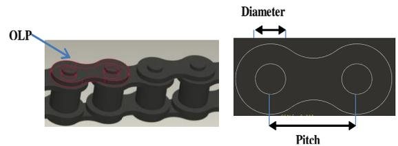
Gambar 3. OLP (Outer Link Plate)
