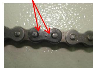
Figure 1. Chain with the distance between the two pins that creep of a standard size
