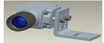
Figure 6. Mechanical design on the CV-020 camera placement
